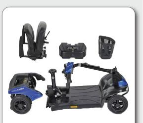
The Colibri is easily dismantled without the need for tools, making it extremely portable
