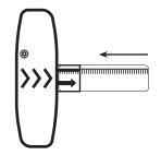
If reactivating the motor is still not effective, a ruler (or similar) can be used to push the pouch out in the direction opposite to normal operation (i.e. towards the start) and removed from the entrance slot. Once the jammed pouch is removed, reset the machine.
