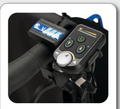
Controller allows you to adjust speed, select forward or backward propulsion and monitor battery level
