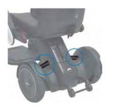
Rear wheel suspension absorbs the impact when driving over bumpy roads or obstacles.
