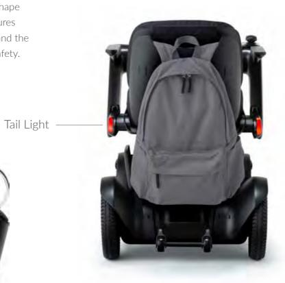
The tail light is clearly visible even with a bag hung over the back support, keeping you safe on the road at night.
