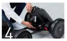
Pull the lever on the side of the battery towards you to separate the parts.
