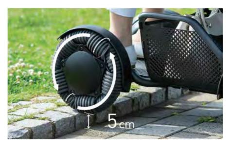
Effortlessly climb over obstacles up to 5cm in height with two powerful motors and large front omni-wheels.
