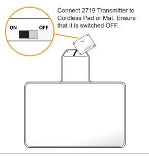
1. Place up to six cordless pads or mats within reach. Each pad or mat must have a 2719 Cordless Pad Transmitter Insert connected & turned OFF.
