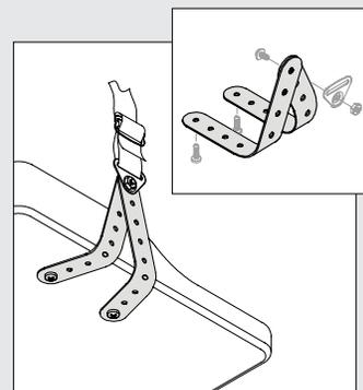
Straps can be bent to attach directly to solid seat bottoms.
