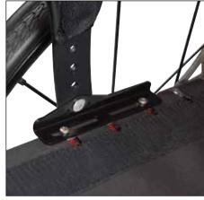
Mounting to the seat rail using Seat Tube Mounting Bracket Kit.
