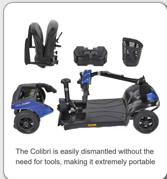
The Colibri is easily dismantled without the need for tools, making it extremely portable
