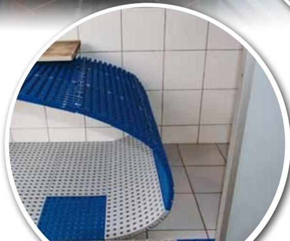
In larger installations, the mat is "rolled up" and rinsed on the underside.
