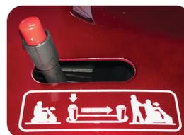
The two-step disengaging lever prevents the scooter from accidentally freewheeling
