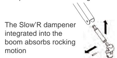
The Slow'R dampener integrated into the boom absorbs rocking motion
