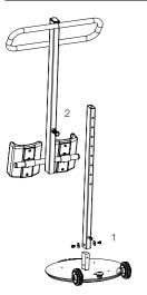
TurnSafe consists of three sections that can be easily disassembled for storage and transport.
