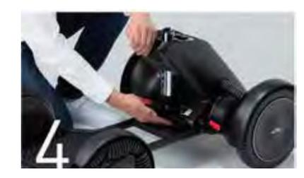
Pull the lever on the side of the battery towards you to separate the parts.
