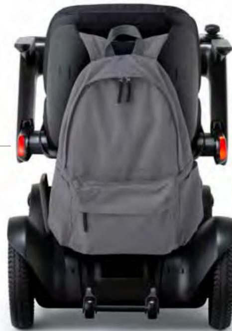
The tail light is clearly visible even with a bag hung over the back support, keeping you safe on the road at night.
